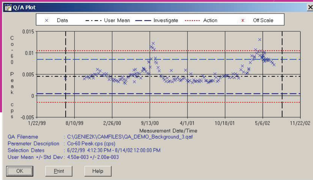
Figure 23 — Representative quality assurance control chart for Co-60 peak area count rate over 3 years. Note the mean, investigate, and action levels displayed.
